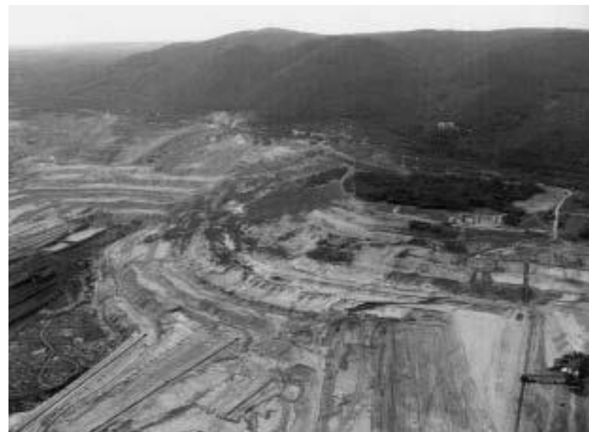
A frontal view of the coal mine in mid-2005, when a massive landslide of about 3 million m 3 of basin sediments was released off the front of the stabilization pillar below Jezeří.
